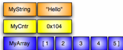
Figure 1: Consider a grouping of data that we might wish to transmit. It has multiple data elements, including a string “MyString”, an integer counter “MyCntr”, and an array of 32-bit unsigned integers called “MyArray”.
